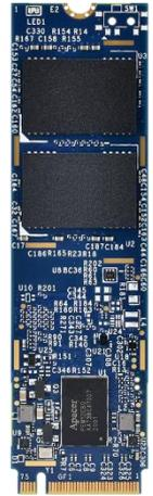
Regarding reliability, PT220-M280 is built with a powerful PCIe controller that supports on-the-module ECC as well as efficient wear leveling scheme. In terms of power efficiency, PT220-M280 is compliant with PCIe Gen3 x4 interface standard so that it can operate on power management modes, which greatly save on power consumption.
