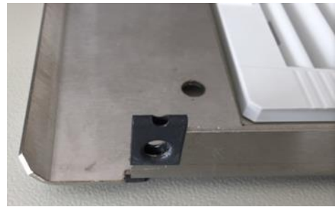
Figure 12: install 4x sheet metal threads
