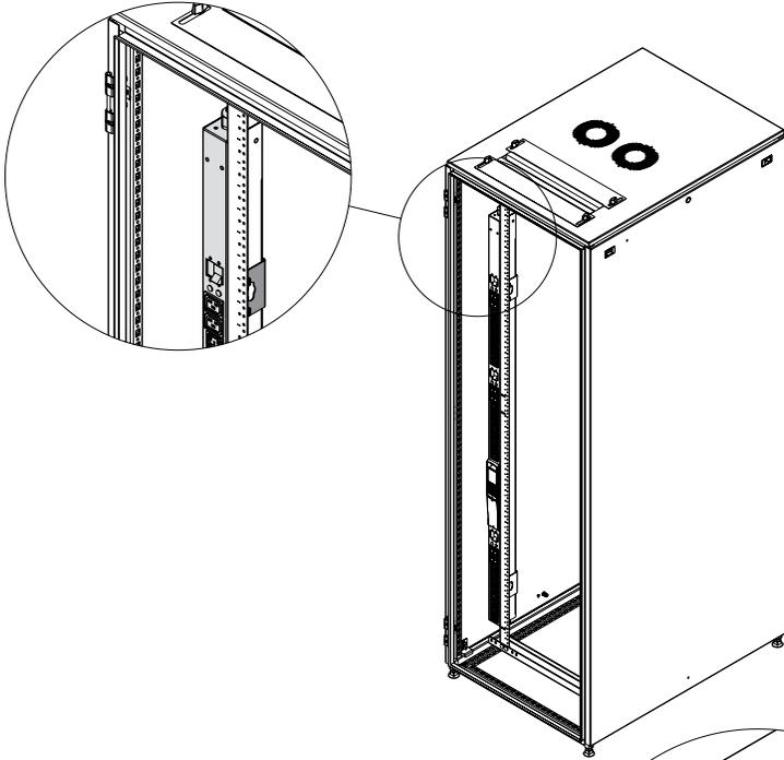
Flush Rack Angle Mount, Dual Feed PDU, Rear Facing
