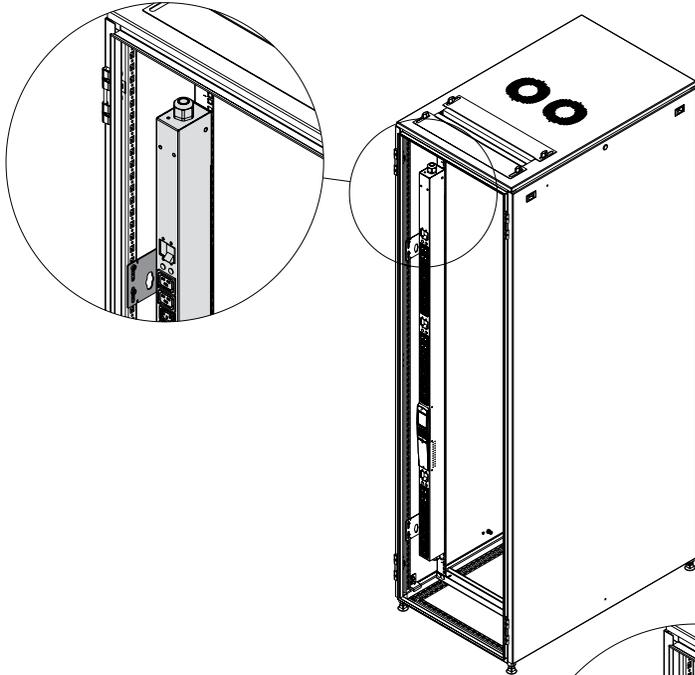
Frame Mount, Dual Feed PDU, Inward Facing
