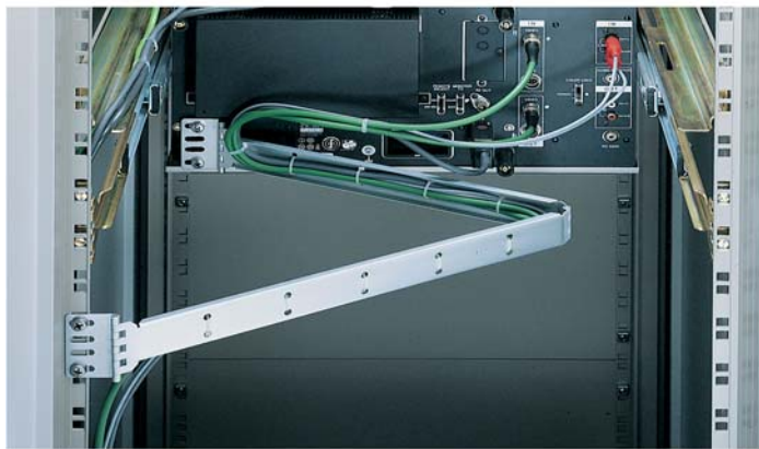
Cable support without return spring
