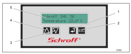
Fig. 18: Control unit (front view)
