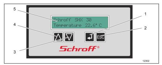
Fig. 9: Control unit (front view)
