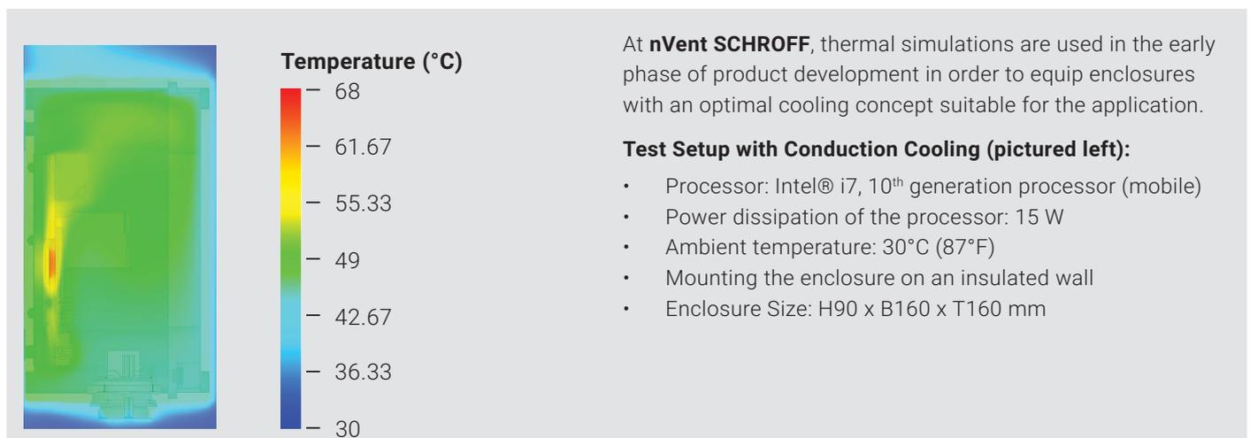
At **nVent SCHROFF**, thermal simulations are used in the early phase of product development in order to equip enclosures with an optimal cooling concept suitable for the application.
