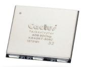
The Cactus Technologies Secure Digital® SDChip (SD) - 806 Series is a low capacity solid-state flash memory product that complies with the Secure Digital Card Association (SDA) standard. Cactus SDChips provide up to 4GB (Class 6) of formatted storage capacity and are designed to be used in applications which require reliable, high performance solid state storage in a high shock & vibration environment.
