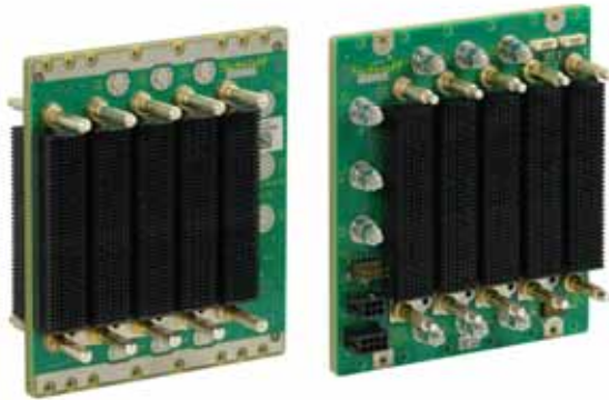
VPX backplane, 3 U, 5 slot, with rear I/O
