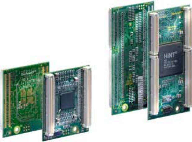
Photo shows 32-bit and 64-bit bridges
