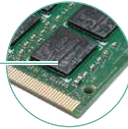
• Apacer DRAM module with conformal coating
