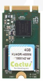
Read Data Transfer Rate : 55MB/s Write Data Transfer Rate : 30MB/s
