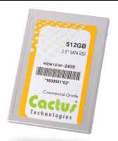
The Cactus Technologies 2.5" SATA III SSD - 240S Series is a high capacity solid state flash memory device which complies with the serial ATA 3.1 specifications, ATA-8 ACS2 command set compatible and can functionally replace a SATA Hard Disk Drive in any application. Cactus Technologies 2.5" SATA III SSDs provide up to 1TB of formatted storage capacity.
