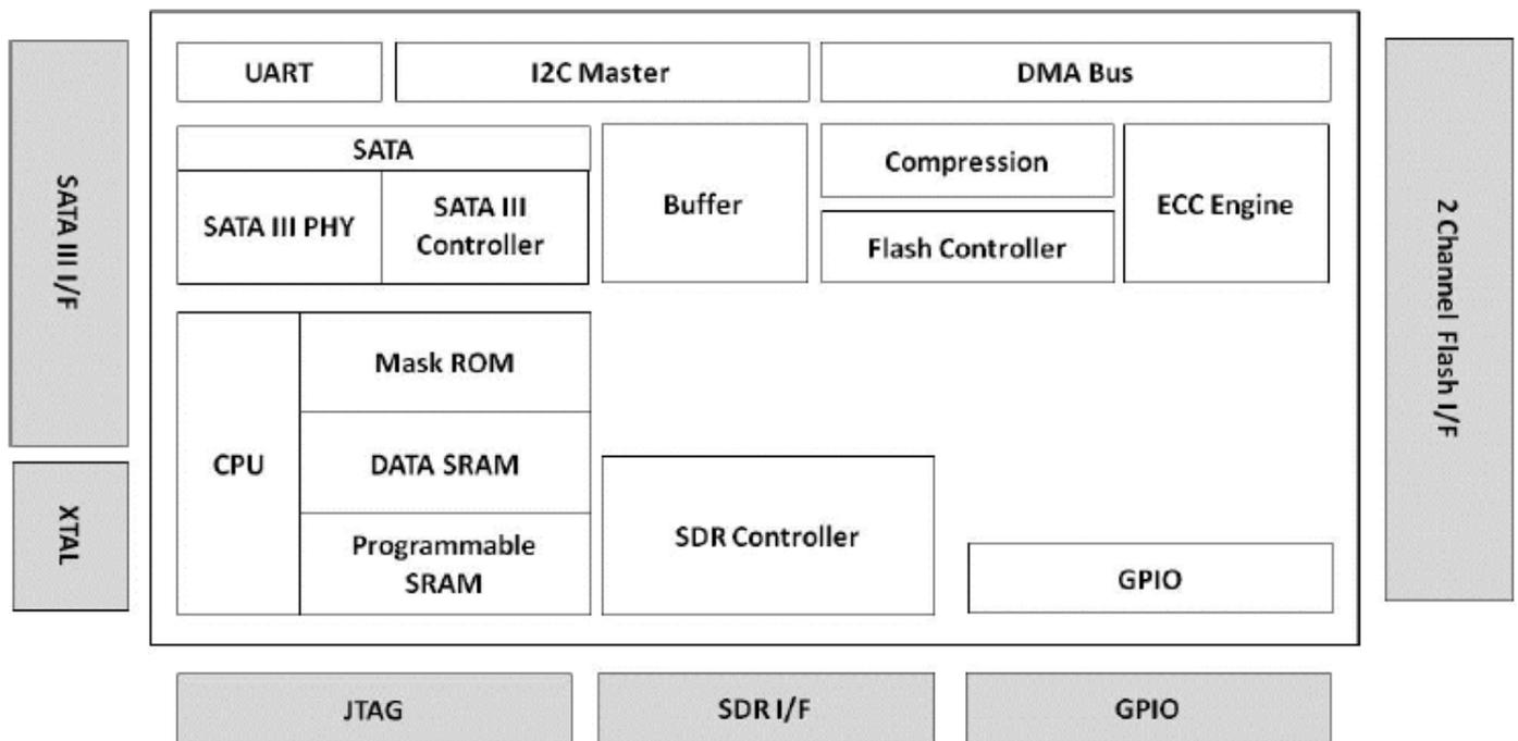
Figure 1: APRO MLC Rugged Metal 2.5" SATA III SSD PHANES-K Series block diagram
