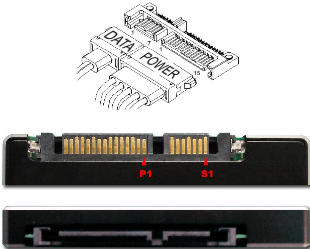
*Figure 3: The connectors of Signal Segment and Power Segment*
