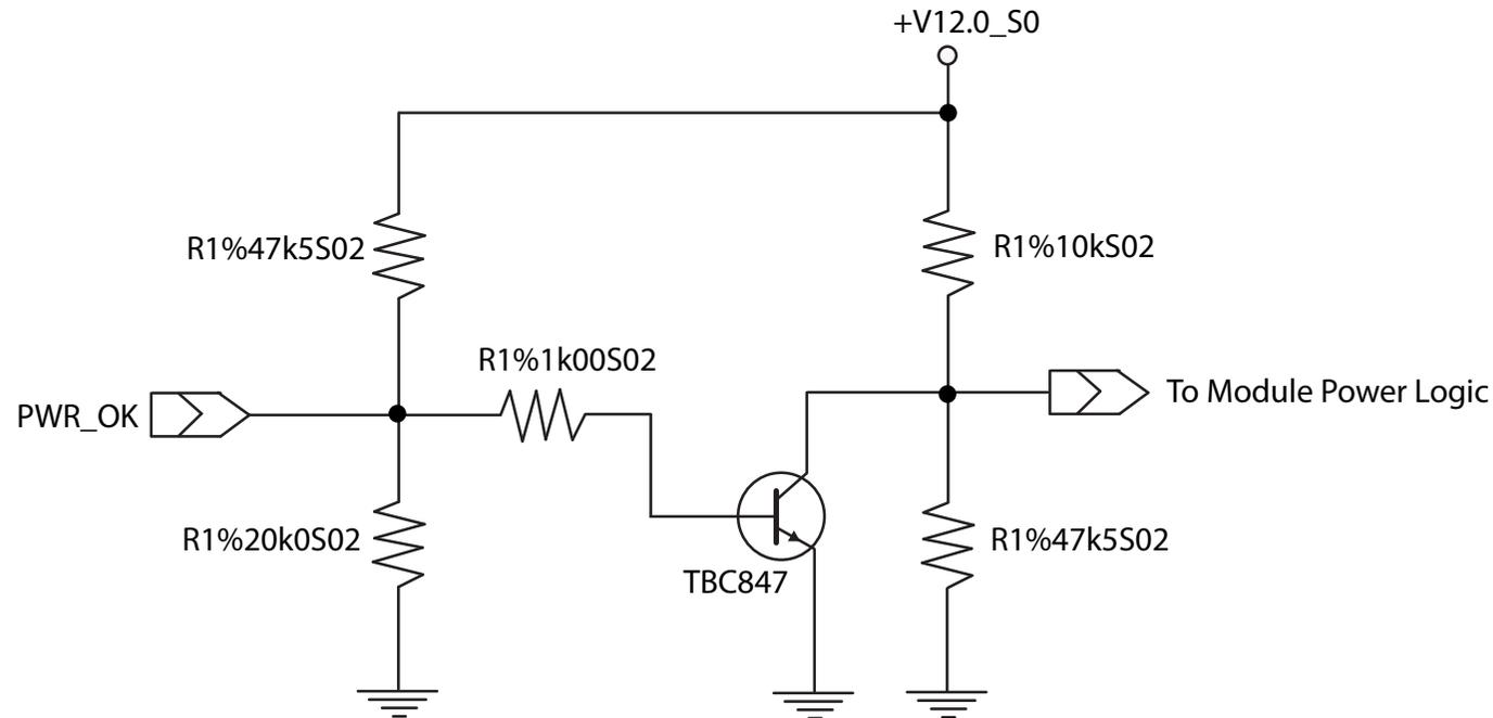
The voltage divider ensures the input complies with 3.3 V CMOS characteristic. It also makes it possible to use the module on carrier board designs that do not use the PWR\_OK signal. Although the PWR\_OK input is not mandatory for the onboard power-up sequencing, it is strongly recommended that the carrier board hardware drives the signal low until it is safe to let the module boot-up.
