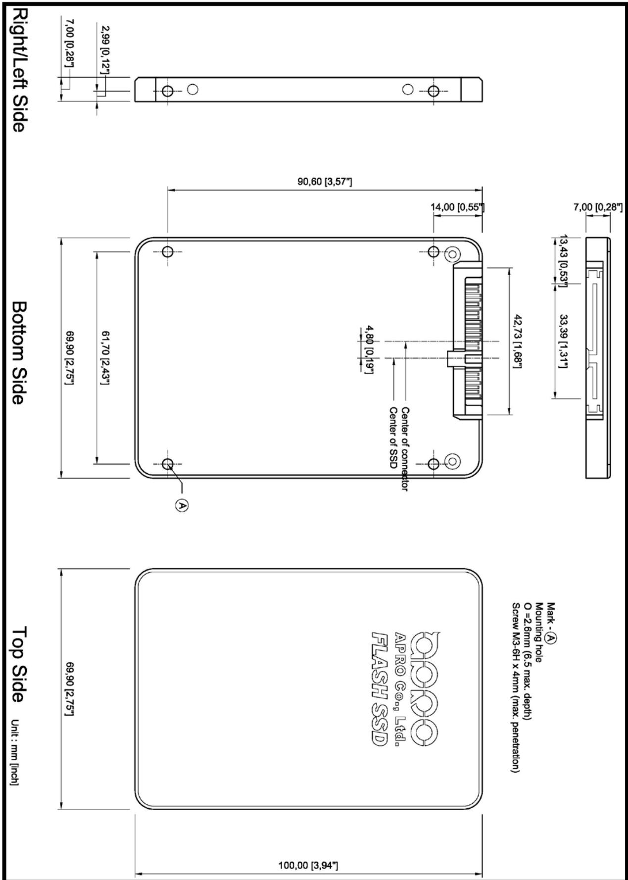
Figure 2: APRO MLC 2.5" Rugged Metal SATA III Flash SSD MUSE-D Series Dimension
