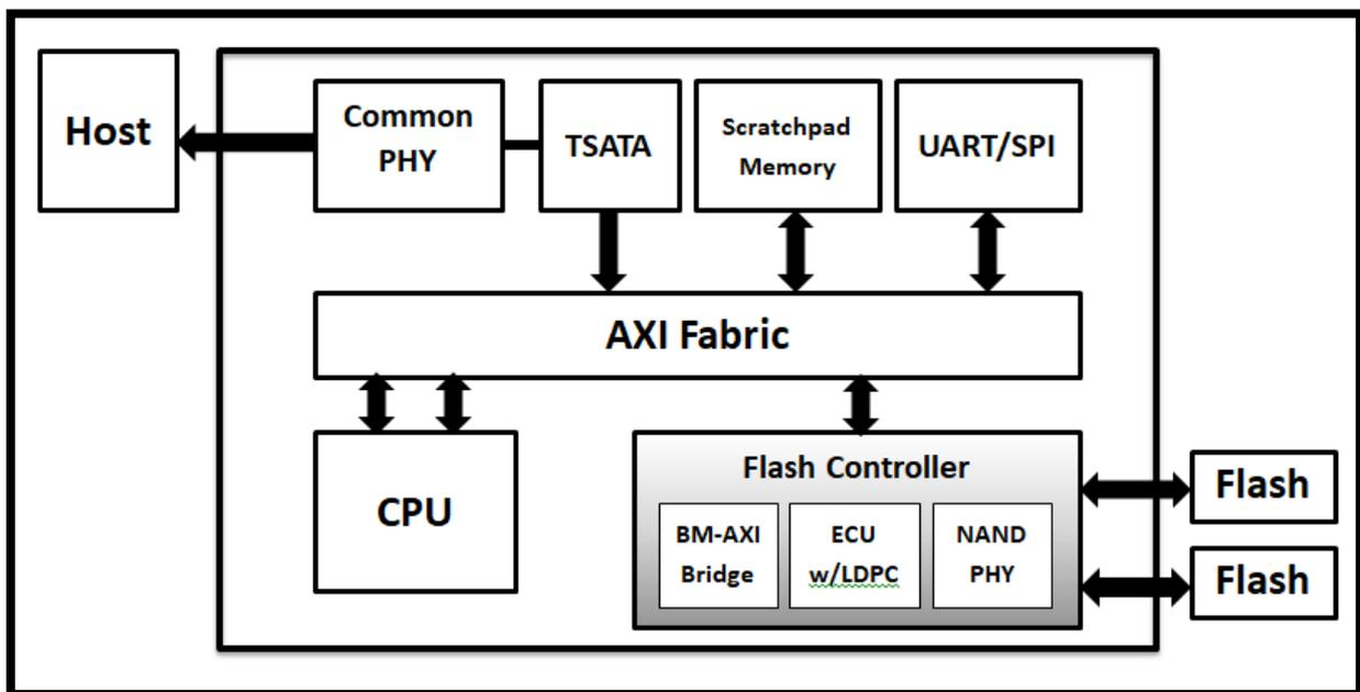
Figure 1: APRO MLC 2.5" Rugged Metal SATA III Flash SSD MUSE-D Series controller block diagram
