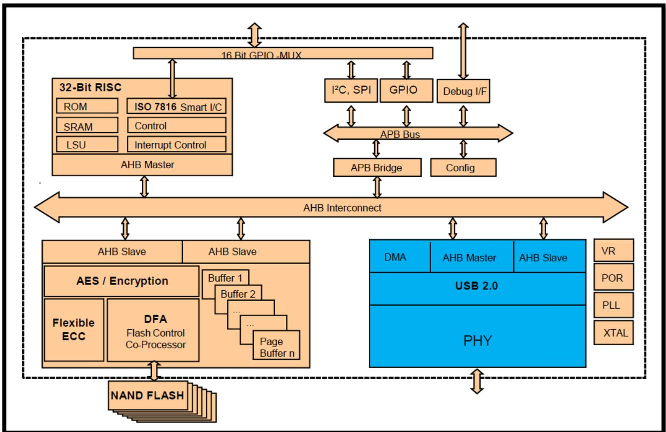
Figure 1: APRO SLC Micro USB Module (MUM) HERMIT-C Series block diagram
