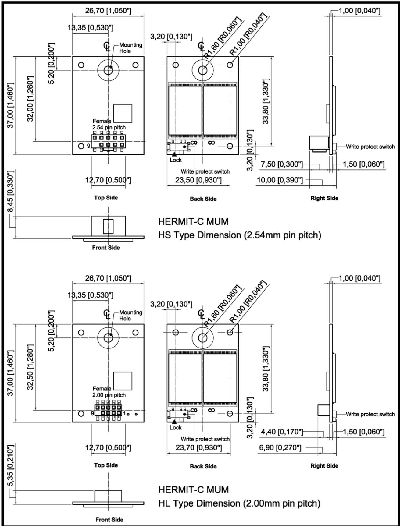
Figure 2: APRO SLC Micro USB Module (MUM) HERMIT-C Series Dimension
