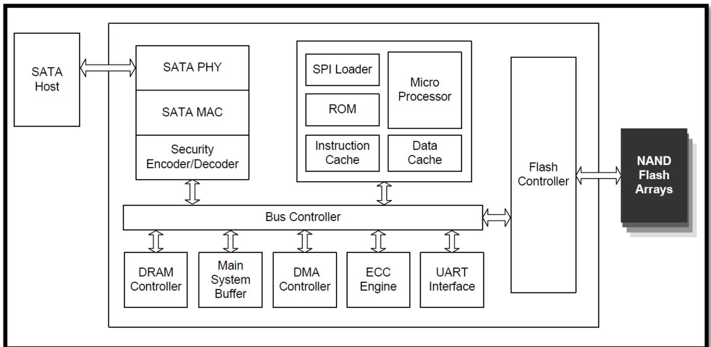
Figure 1: APRO SLC Industrial 2.5" Rugged Metal SATA III SSD HERCULES-TR Series block diagram
