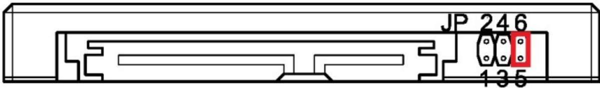
Figure 8: Write-Protect Function Jumper Setting
