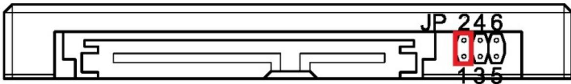
Figure 5: Fast Erase Jumper Setting
