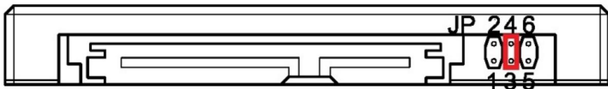
Figure 6: Secure Erase Jumper Setting
