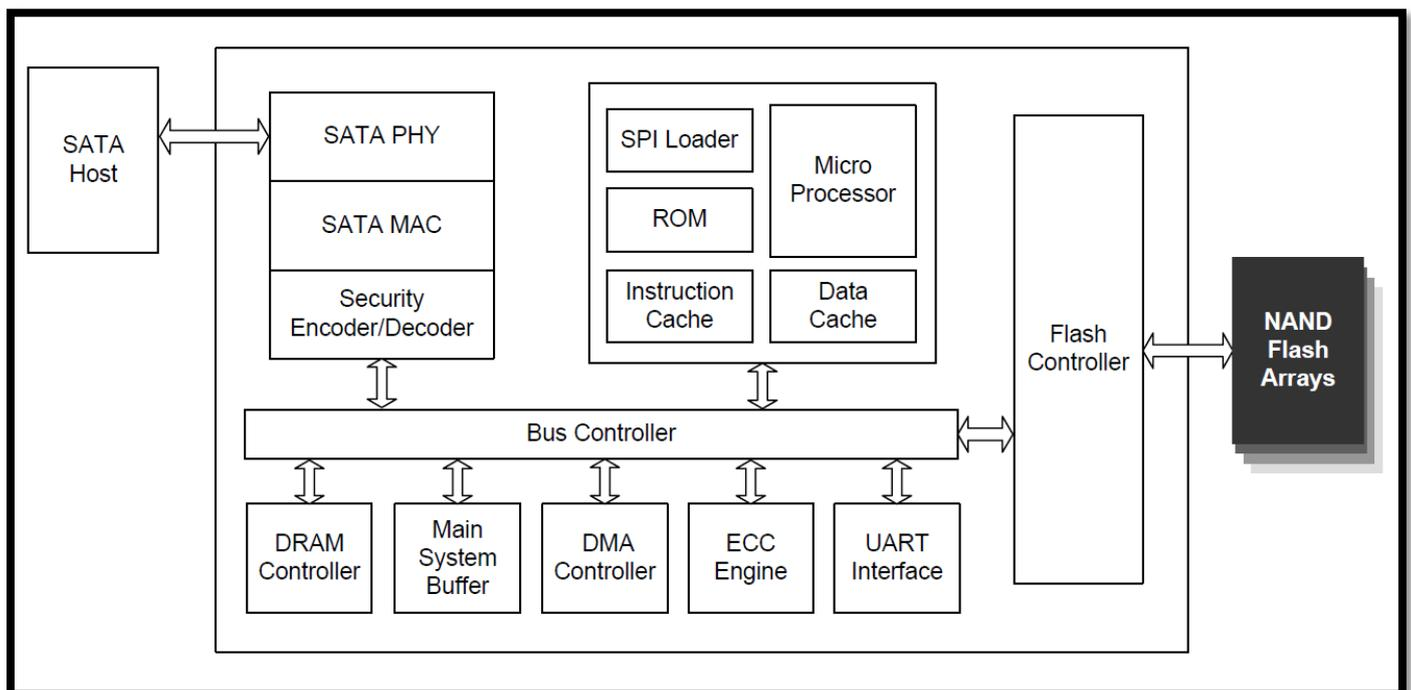
Figure 1: APRO SLC Industrial 2.5" Rugged Metal SATA III SSD BON-III series block diagram
