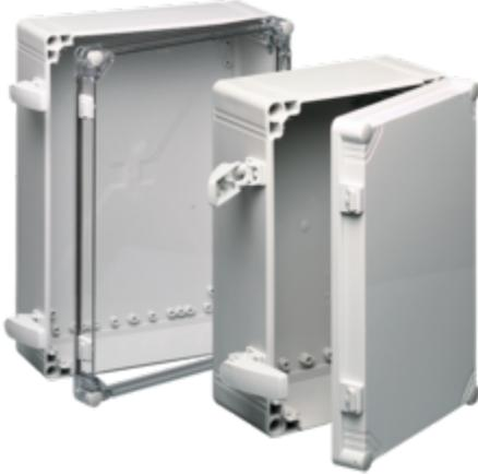
The largest-sized QLine enclosure, QLine I provides easy access and protects larger controls from corrosive environments. Choose from screw cover, hinge, internal mounting, variable depth and quick-release latch options to meet your design and security requirements. The ABS series shares the same features and similar physical properties as the polycarbonate but is a more economical, non-UL rated alternative.
