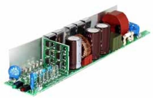
Application: DC/DC converter for supply power to fans (with monitoring) 11309005
