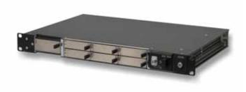
MicroTCA system, 1 U for 6 single mid-size AMC modules; power supply, increased air inlet and exhaust area with inwardly curved side panels
