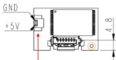
For external power cable connection: this feature is available as an option for Standard Type.
