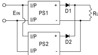
2. When using S.P.S. in parallel connection, the leakage current will increase at the same time. This could pose as a shock hazard for the user. So please contact the supplier if you have this kind of application.
