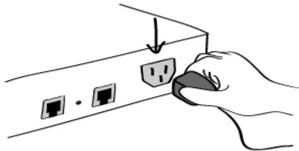
*Figure 2-4 Connecting the power to the STS1600*
