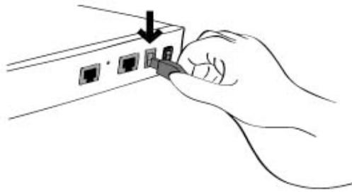
*Figure 2-3 Connecting the power to the STS400/800*
