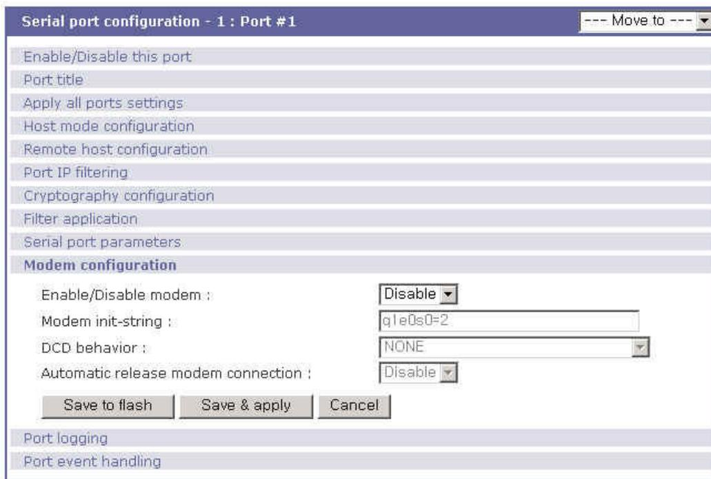
Figure 4-16 Modem configuration
