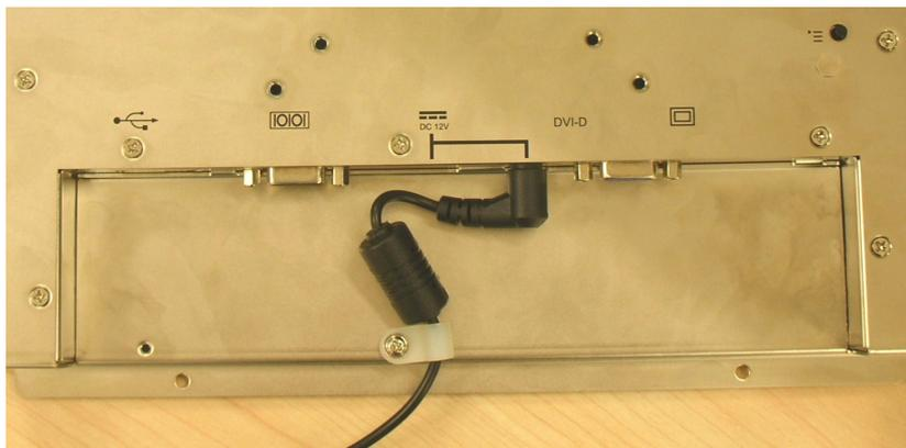
2. A cable tie for the USB cable is included in the accessory box, see below:
