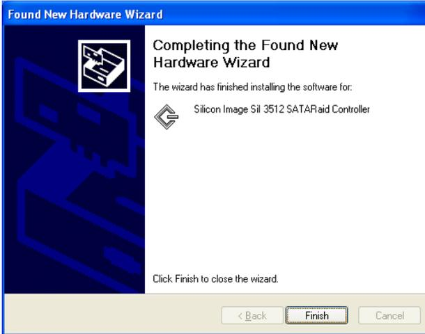
7. You can find the file “**Silcon Image Sil 3512 SATA RAID Controller**” in **Device Manager**, and you’ve done installing the PER-C20S driver
