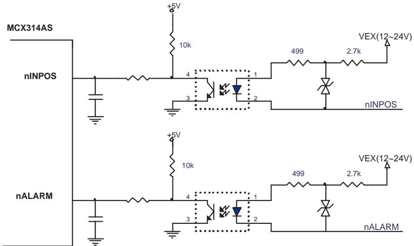
**Figure 3.10: Input Signal for Servo Motor**
