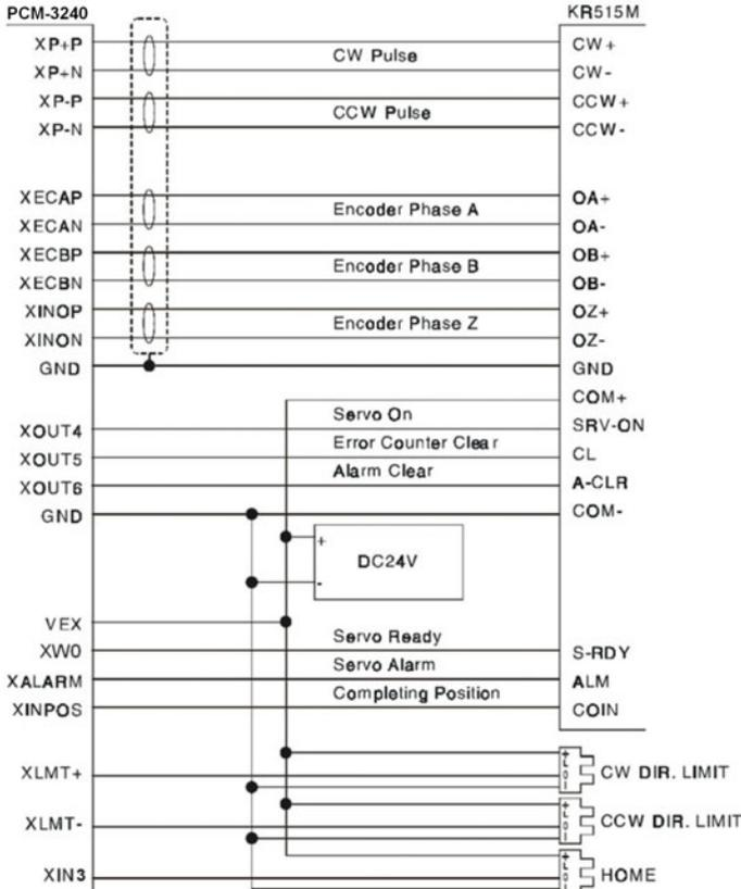
**Figure 3.20: Connection Example to MINAS X series AC servo motor drive**
