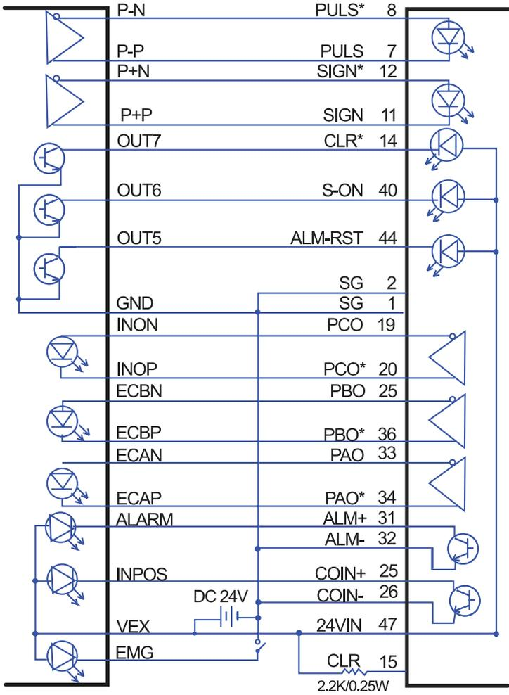
**Figure D.4: Wiring Diagram with Yaskawa SGDM Series Motor Driver**
