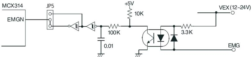
**Figure 3.16: Circuit Diagram of Emergency Stop Input Signal**
