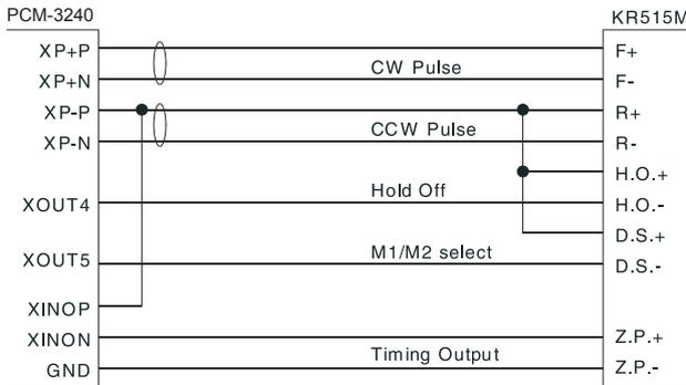
**Figure 3.18: Example of connecting to KR515M drive**
