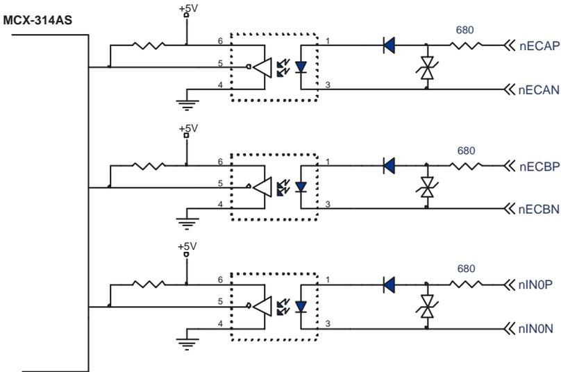
**Figure 3.11: Circuit Diagram of Encoder Feedback**
