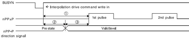
**Figure 3.22: Timing diagram of Individual Axis Driving**
