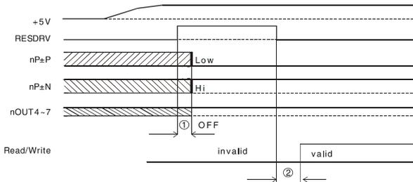
**Figure 3.21: Timing diagram of Power On RESET**
