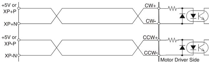
**Figure 3.4: Photo coupler input interface**
