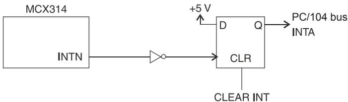
**Figure 3.17: Circuit Diagram of Interrupt Setting**
