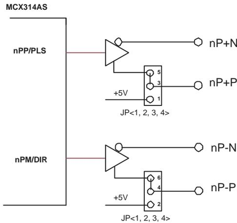
**Figure 3.3: Output Signal Loop for Drive Pulses**
