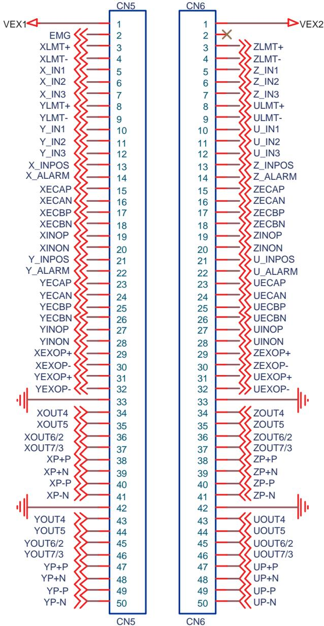
**Figure 3.1: I/O Connector Pin Assignments for the PCM-3240**
