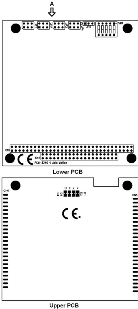
**Figure 3.2: Location of Jumpers and DIP switch on PCM-3240**
