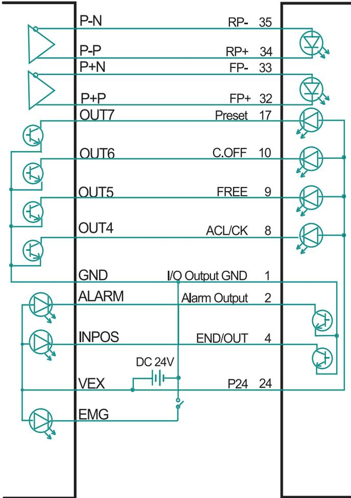
**Figure D.2: Wiring Diagram with Oriental LIMO EZMC Series Motor Driver**
