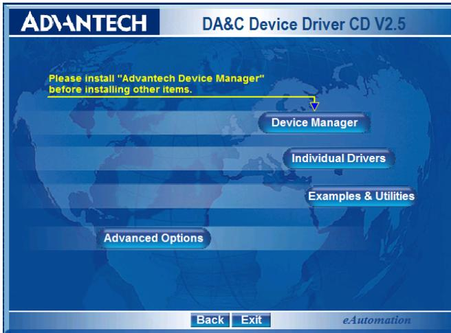
**Step 5:** Please install the ‘Device Manager’ first. For details on how to install the ‘Device Manager’ step by step, please see the software manual.
