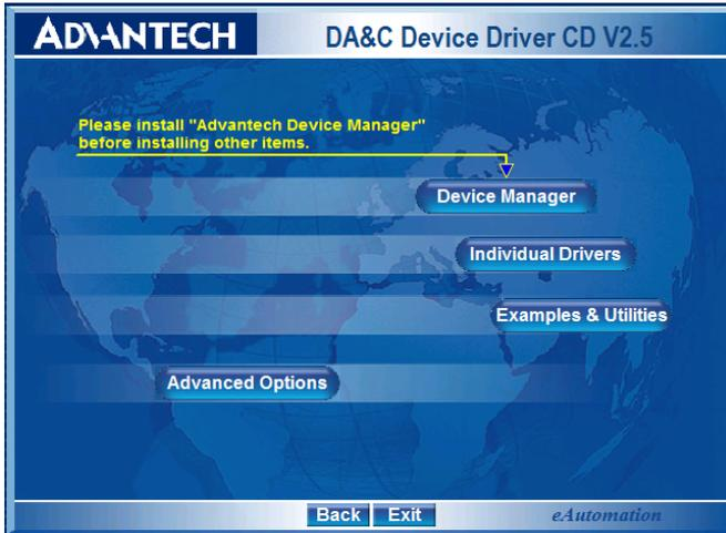
**Step 6:** When you’re finished installing the ‘Device manager’, you can install the driver of the corresponding card. Please click the ‘Individual Drivers’
