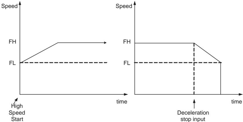
**Figure 4.1: R4's Effect on Output Pulse Speed**
