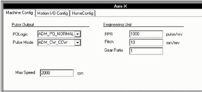
*Figure 3.4: Machine Configuration Page*
