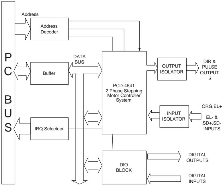
**Figure 1.1: PCI-1243U 4-Axis Stepping Motor Control Card**
