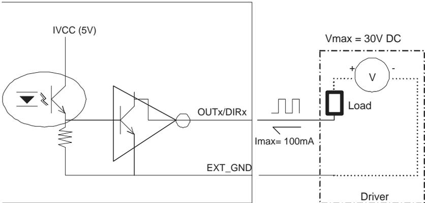
**Figure 2.3: Pulse Output Test Configuration (Open Collector Type)**
