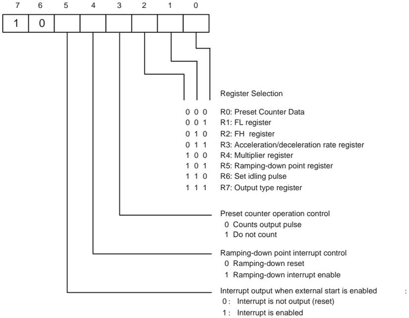
Register select code: Selecting an access register with last 3 bits.
