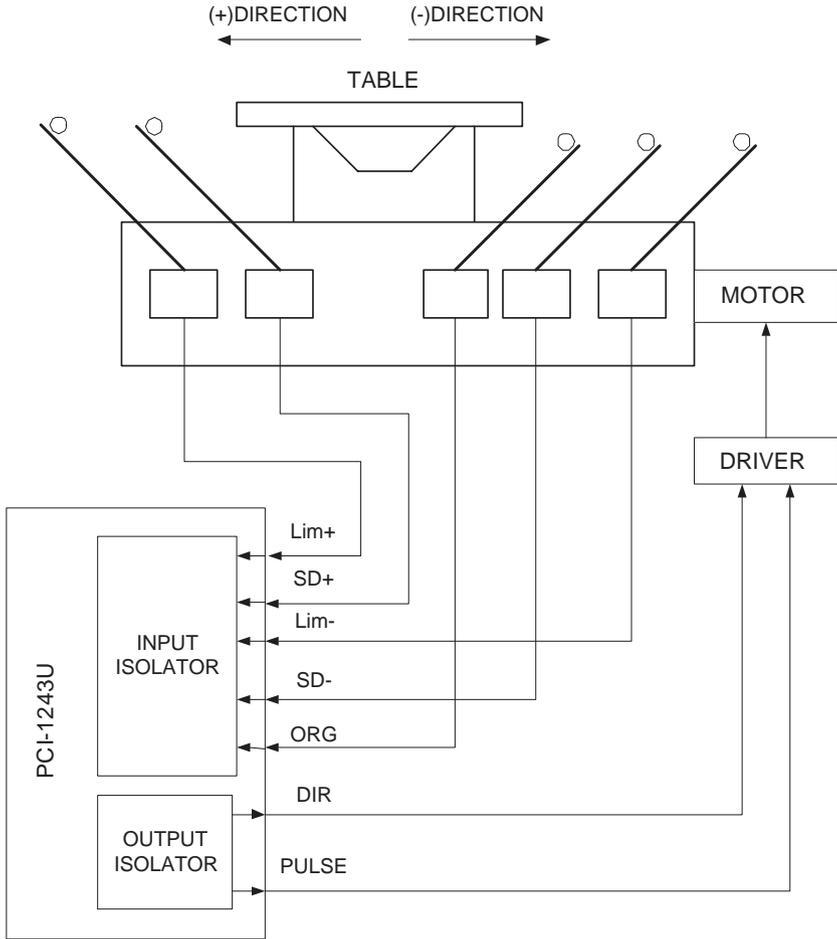
*Figure 2.6: Limit Switches*
