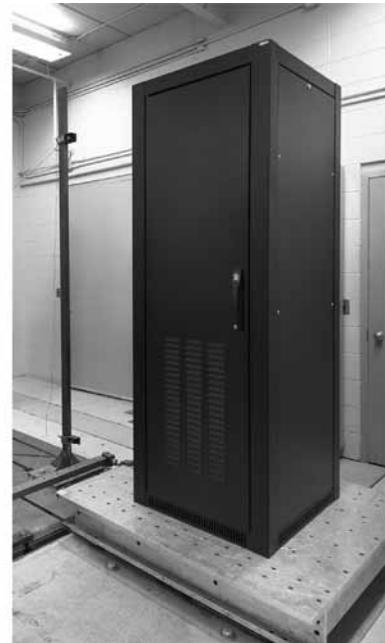
*Enclosure mounted on shaker table*
