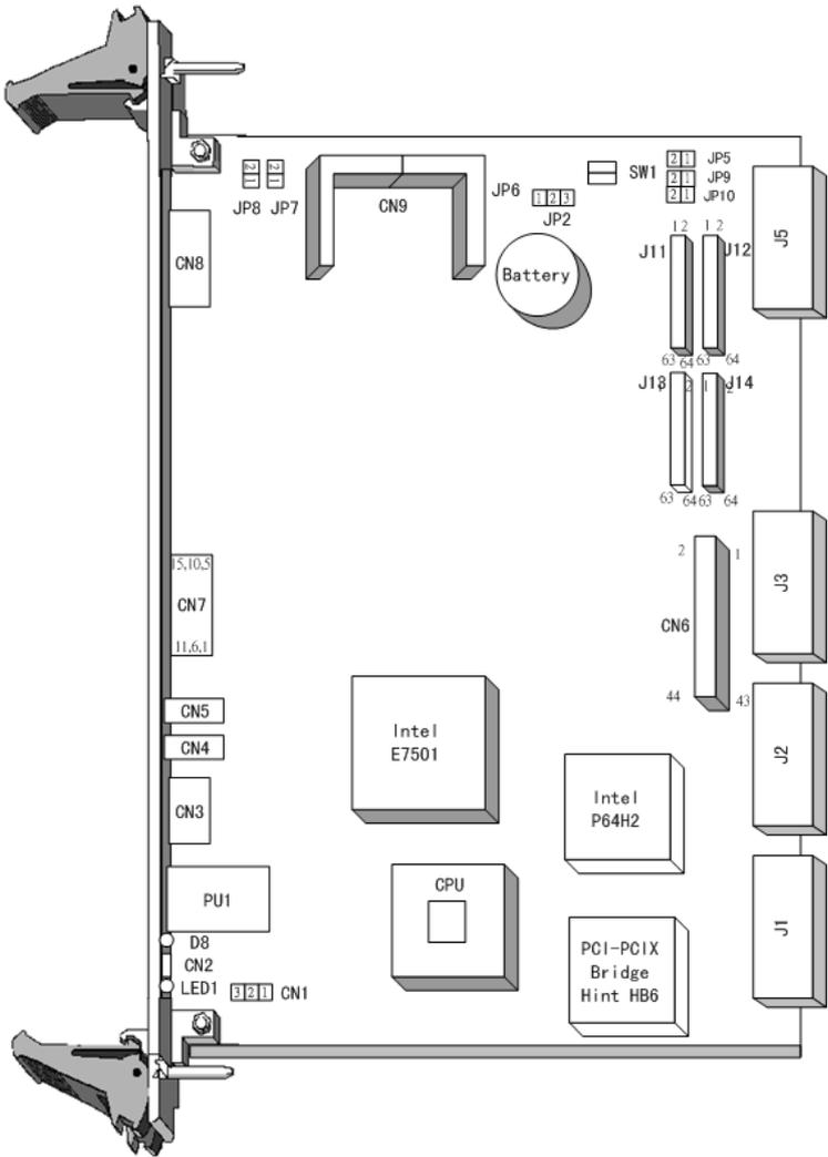
**Figure 1.3: MIC-3369C Jumper and connector locations**
