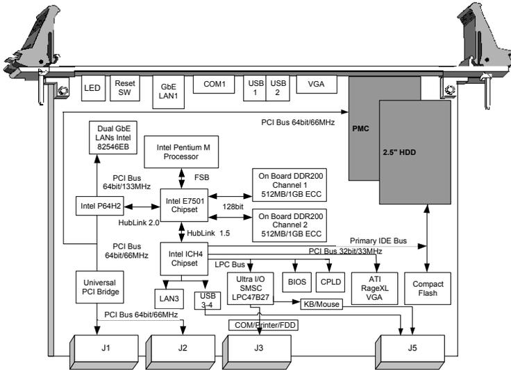
**Figure 1.1: MIC-3369C functional block diagram.**
