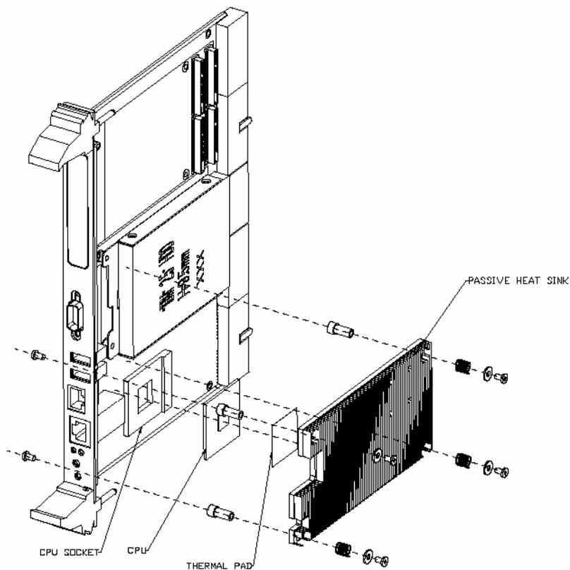
*Figure 1.5: Complete assembly, heatsink and HDD*
