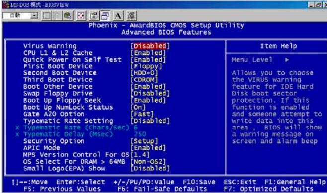
Figure 4.3: Advanced BIOS features setup screen
