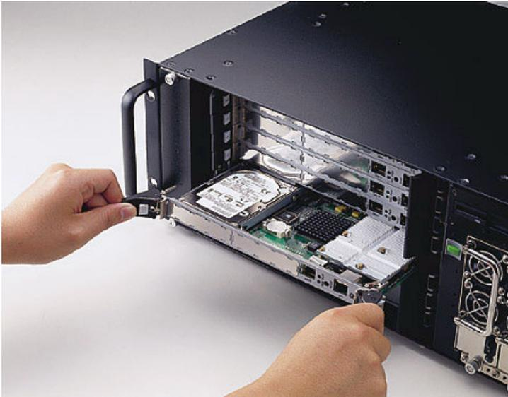
***Figure 2-3: Installing a card into the chassis***
