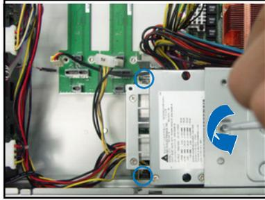
4. Carefully lift the power supply cage upward a little to remove it from the chassis.
