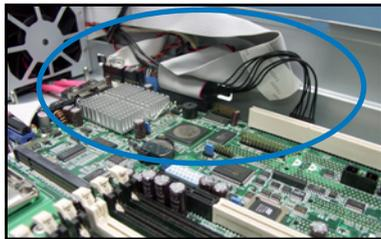
8. Take note of the two pegs on the Riser cage bay. These pegs should match the holes on the cage to make sure it fits in place.
