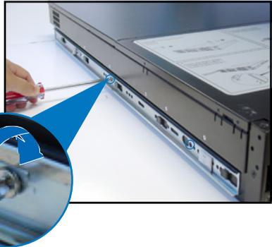
4. Repeat steps 1 to 3 to attach the second server rail to the other side of the chassis.
