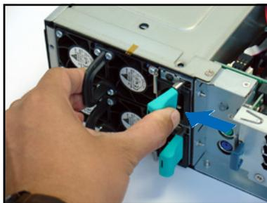
3. Firmly pull the lever to slide the power supply module out of the chassis.
