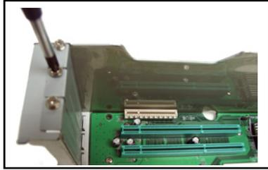
4. The card golden connectors should match the notches on the slot. Then, firmly push down the card until it is completely seated on the slot.
