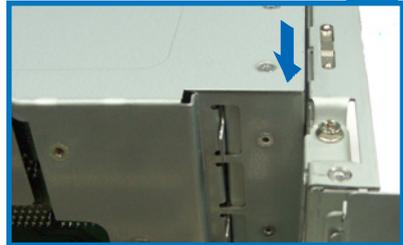
10. Match and push the cage card connector into the PCI-E slot until the PCI cage fits in place.
