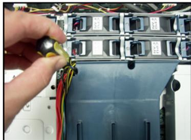
6. When the air duct is in place, arrange the power cable cluster to fit the space beside the air duct.
