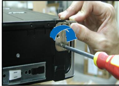
4. Pull the server rail lock, then push the server all the way to the depth of the rack. Make sure that the mounting ear and the rack screw holes align.
