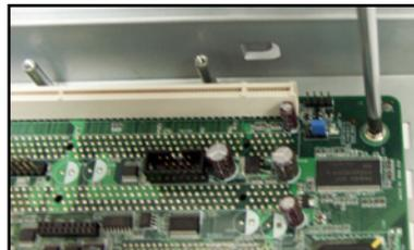
4. After installing the riser card with a ZCR card, fasten the screw back..
