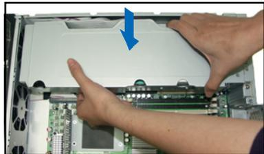
11. Ensure that the golden connectors of the riser cage card completely fit the slot. If properly installed, the top of the PCI cage aligns with the top edge of the rear panel.
