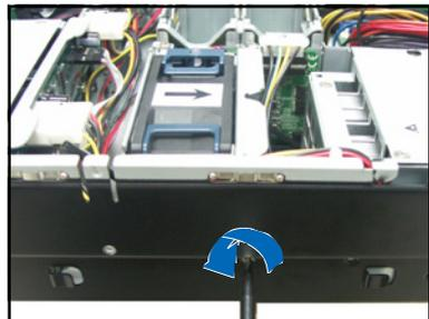
2. Remove all the fans and unscrew the fan rack.
