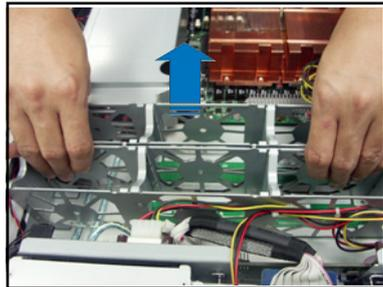
6. Unscrew the mid-fan board and remove it from the fan rack.
