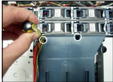
3. Hold the rear part of the air duct and press it for about a fraction of an inch, just enough to tilt the front end. When tilted, carefully pull the air duct upward to release it from the chassis.
