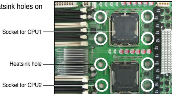
2. Position the CEK spring underneath the motherboard, then match the CEK spring hooks to the CPU1 heatsink holes.
