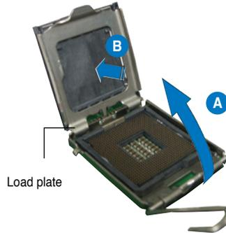
5. Position the CPU over the socket, making sure that the gold triangle is on the bottom-left corner of the socket. The socket alignment key should fit into the CPU notch.
