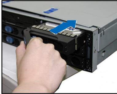
7. Push the tray lever until it clicks, and secures the drive tray in place. The drive tray is correctly placed when its front edge aligns with the bay edge.
