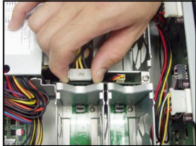
4. Remove rack fan for the power supply first and then loosen the screw that fastens the fan rack to the power supply cage.
