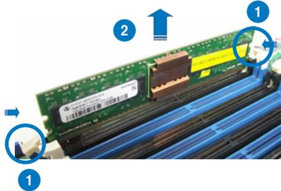
2. Remove the DIMM from the socket.
