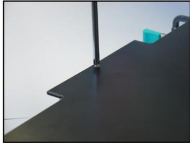
3. Firmly hold the rear half of the top cover, then remove it from the chassis.
