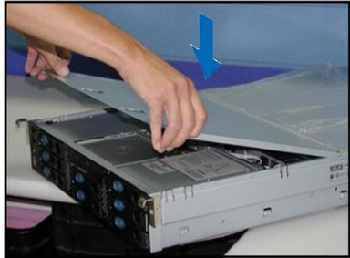
4. Push the sliding locks toward the front edge to secure the front half of the top cover in place.
