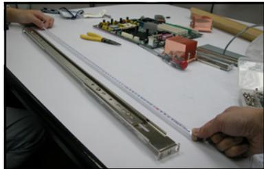
8. Position the rack rail to the 2U space on the rack. Make sure that the front end of the rack rail goes to the front of the rack space.
