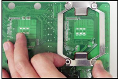
5. If you installed a second CPU, repeat steps 2 to 4 to install the CEK spring to the CPU2 heatsink holes.
