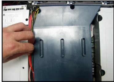
2. Loosen the two screws that fasten the air duct.
