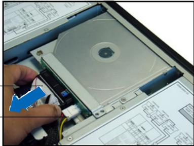
2. Loosen the two screws that secure the drive bracket to the chassis. The optical drive is attached to the top of the bracket, and the floppy drive to bottom.
