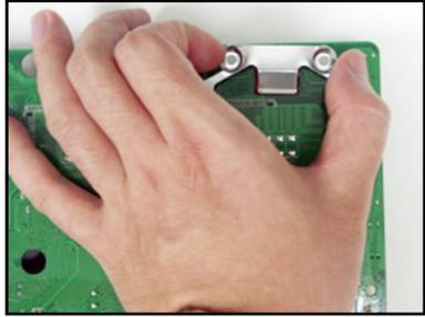
4. Press the lower spring clips inward, then insert to the lower CPU heatsink holes until they snap in place.
