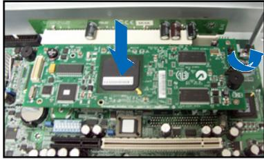
5. Align the other support bracket for the ZCR card to the screw holes on the chassis.
