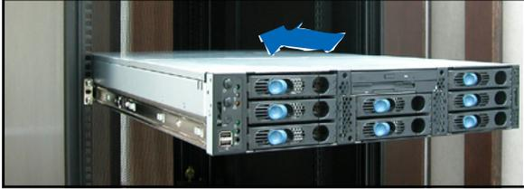
2. Align a mounting ear with the holes on a front corner of the chassis, then secure it with two screws.
