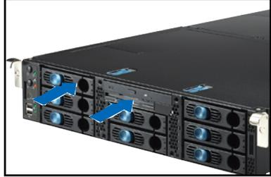
2. With both hands, flip up the front corners of the top cover, then lift. The front corners of the cover have dents that match those on the chassis. These dents provide a holding mechanism and keeps the cover in place even when the sliding locks are released.
