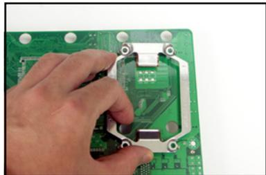
3. Press the upper spring hooks inward, then insert to the upper CPU heatsink holes until they snap in place.
