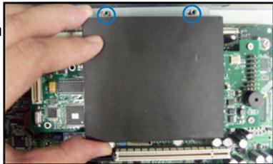
6. Secure the support bracket for the ZCR card with screws.
