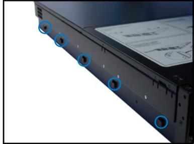
2. Position a server rail parallel to the side of the chassis, and match each of the five hooks to the holes on the rail.
