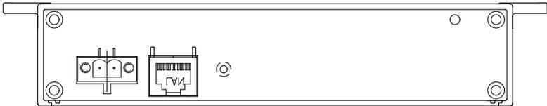
**Figure 2.9: EDG-4504—Front Panel**
