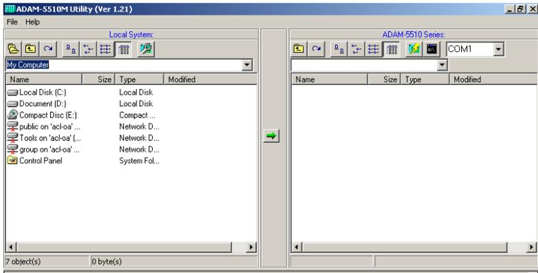
2. Click the refresh button to check if the drive D: of ADAM-5510TCP is detected correctly.
