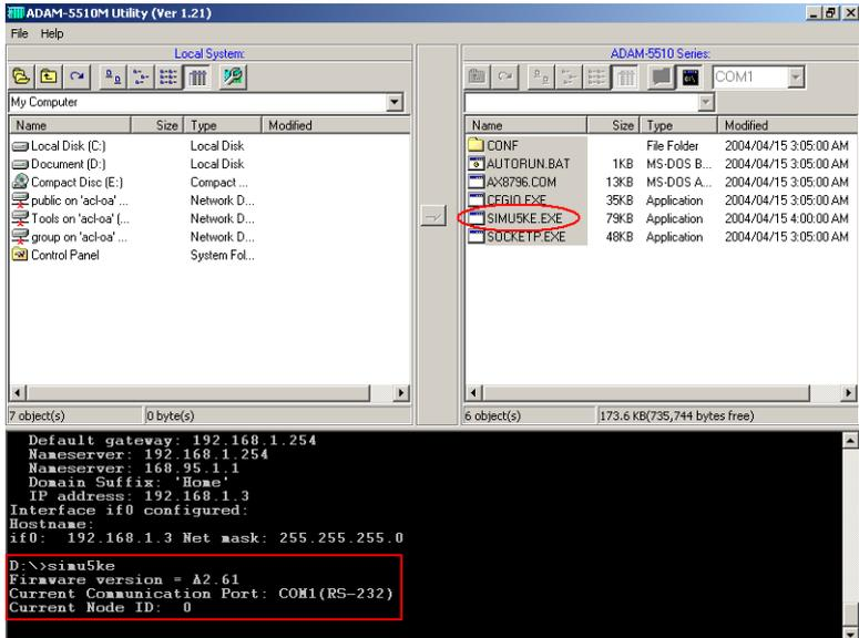
8. Connect the Host PC to COM1/RS-232 on ADAM-5510/TCP by a null modem cable.
