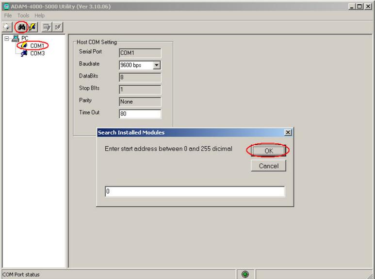
11. Search the ADAM-5510/TCP Module and configure the input range of the ADAM-5017 Analog Input Module.
