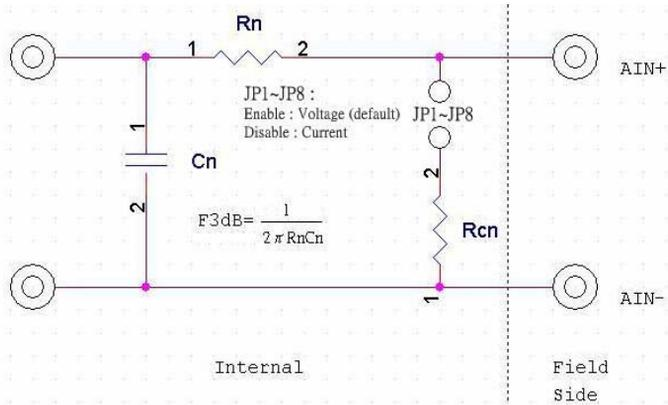
Figure 14: Locations of RC Filter Jumper setting
