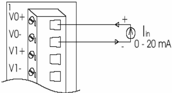
*Figure 13: Process current input*
