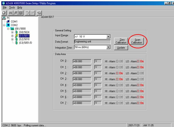
*Figure 24: Span calibration*
