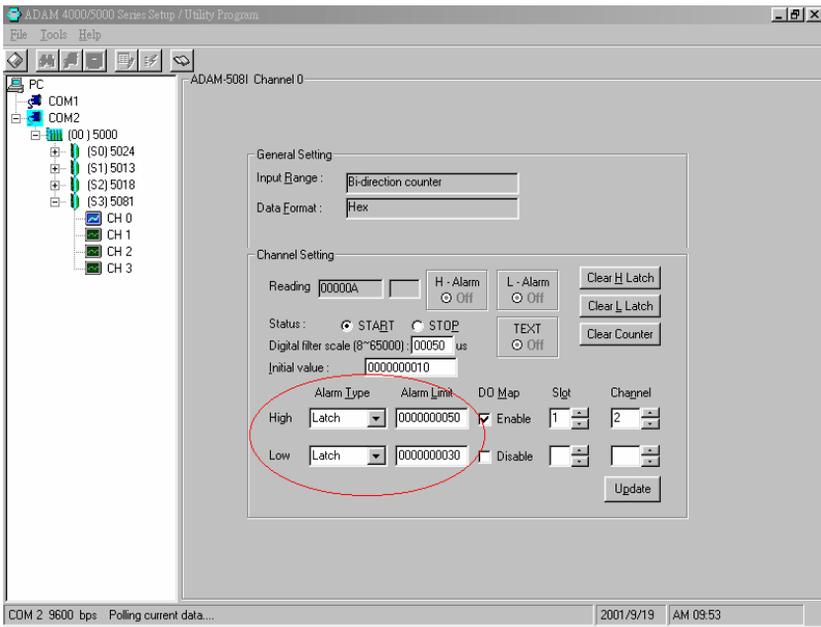
Figure 59: Setting Alarm Limit
