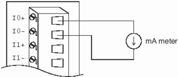
*Figure 26: Output module calibration*
