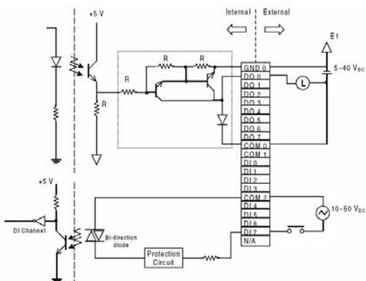
Figure 40: ADAM-5055S module wiring diagram
