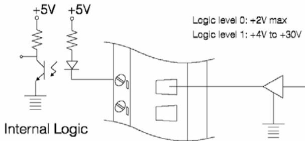
*Figure 30: Wet contact signal input (ADAM-5050)*
