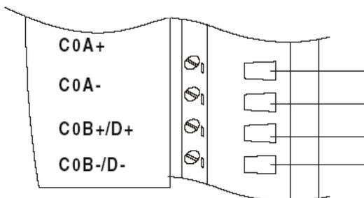
*Figure 57: Wiring for Bi-direction Counting*
