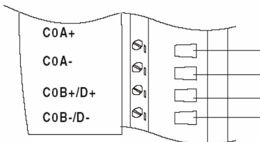
*Figure 56: Wiring for Up/Down Counting*
