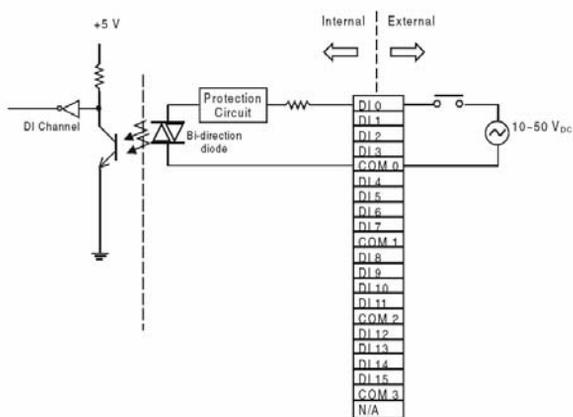
Figure 36: ADAM-5051S module wiring diagram
