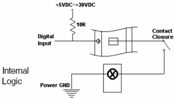
*Figure 34: Contact closure input (ADAM-5051/5051D)*
