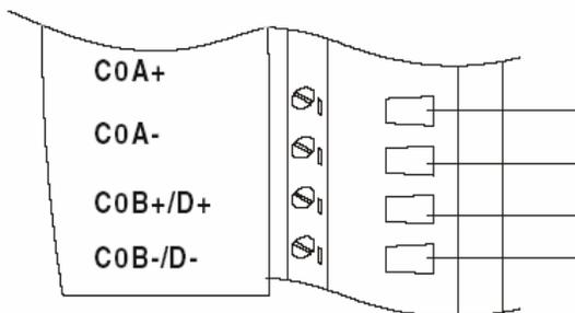
*Figure 56: Wiring for Up/Down Counting*
