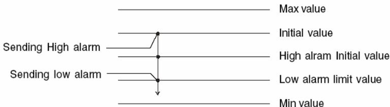
*Figure 61: Sending Alarm Signal (settings not recommended)*
