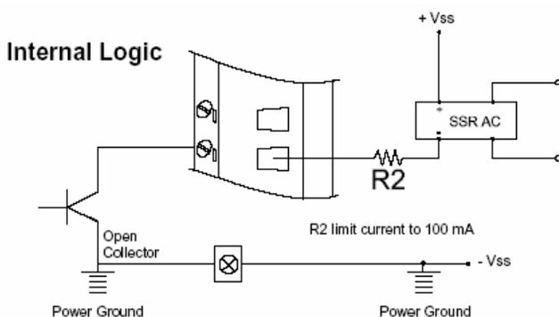
Figure 42: Digital output used with SSR (ADAM-5050/5056)
