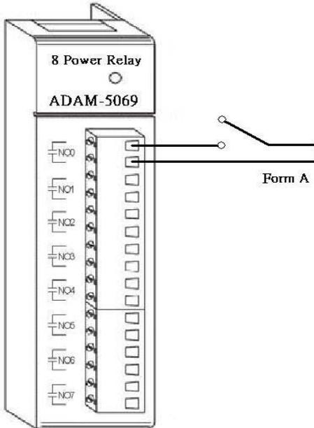
*Figure 51: the wiring of ADAM-5069 module frontal view*
