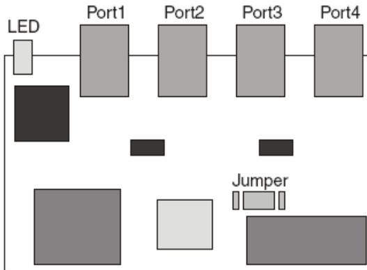
*Figure 67: Jumper locations on the CPU card*
