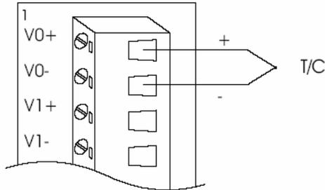
*Figure 19: Thermocouple input*
