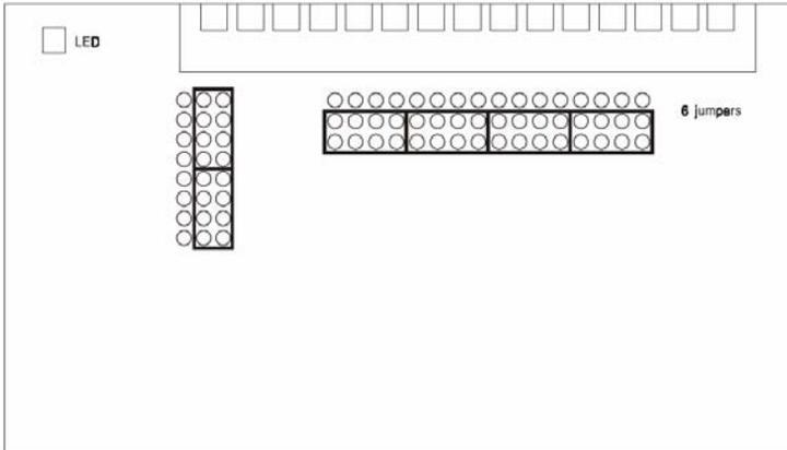
*Figure 63: Jumper Location on the ADAM-5080 Module*
