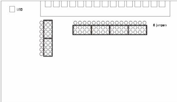
*Figure 63: Jumper Location on the ADAM-5081 Module*
