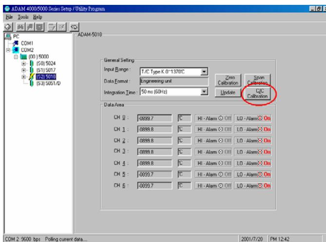
**Figure 25: Cold junction calibration**
