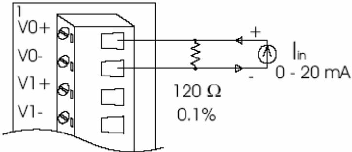
*Figure 9: Process current input*
