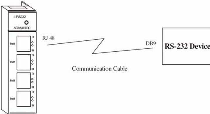
Figure 66: ADAM-5090 Application Wiring
