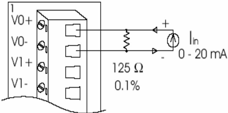
*Figure 6: Process current input*
