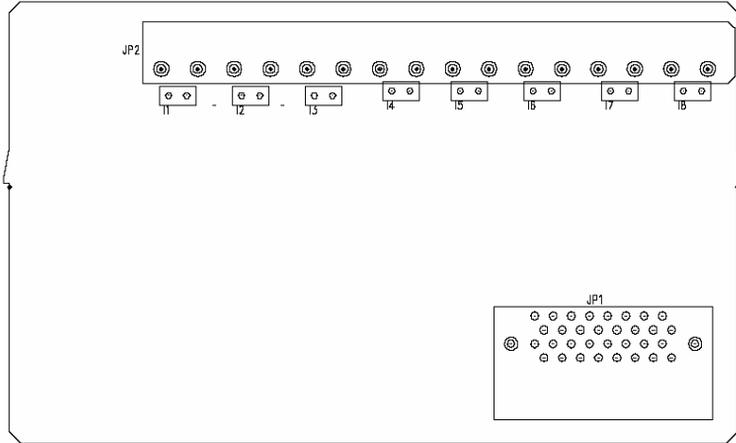
*Figure 13: Locations of 125-ohm resistors*
