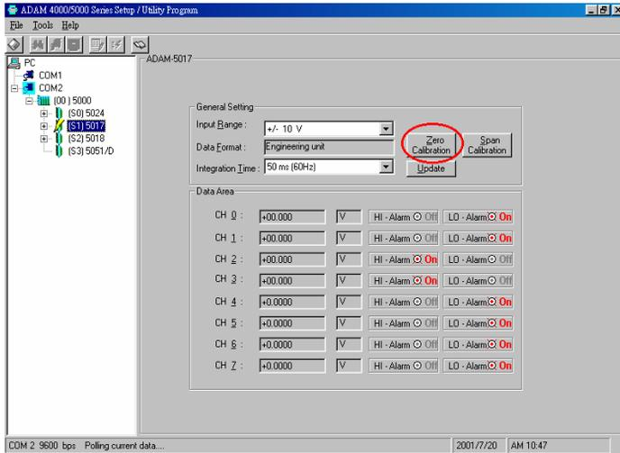
*Figure 23: Zero calibration*
