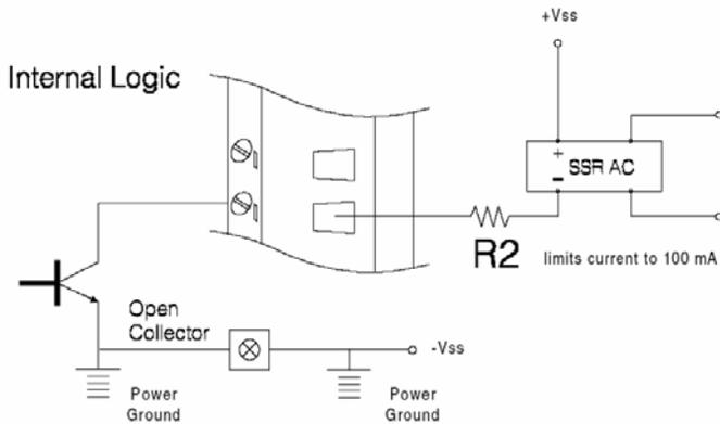
*Figure 31: Digital output used with SSR (ADAM-5050/5056)*
