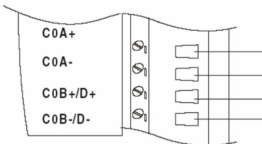
*Figure 57: Wiring for Bi-direction Counting*
