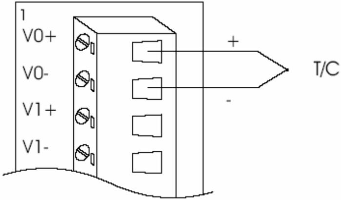
*Figure 17: Thermocouple input*
