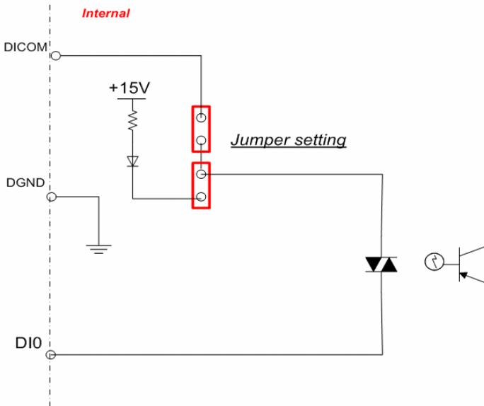
**Figure 3-56a ADAM-4055 Default Jumper Setting for the Digital Input Wiring**
