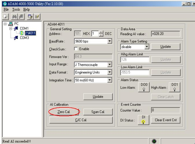
**Figure 8-2 Zero Calibration**
