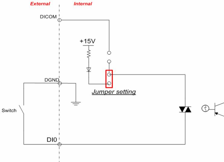
**Figure 3-54b ADAM-4055 Digital Input Dry Contact Diagram (Internal)**
