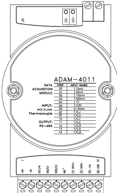
Figure 3-1 ADAM-4011 Thermocouple Input Module
