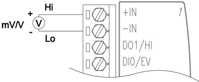
Figure 3-4 ADAM-4011/4011D Millivolt and Volt Input Wiring Diagram
