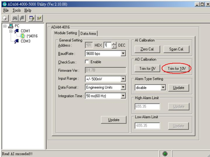
**Figure 8-9 Span Calibration**
