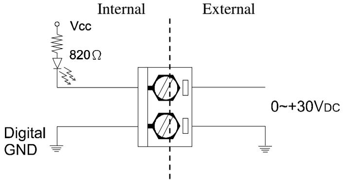
Figure 3-50 ADAM-4053 Wet Contact Input Wiring Diagram
