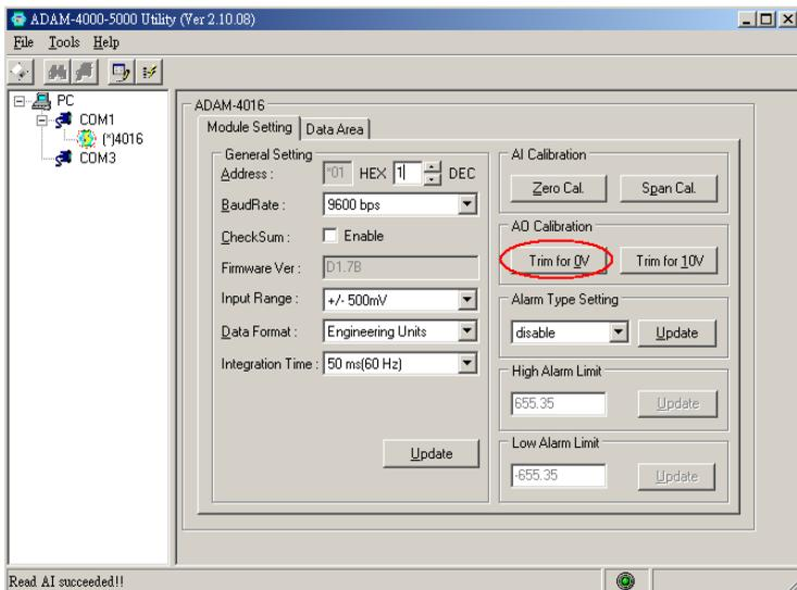
**Figure 8-8 Zero Calibration**
