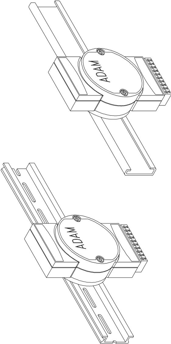
**Figure C-3** *DIN-Rail Mounting*
