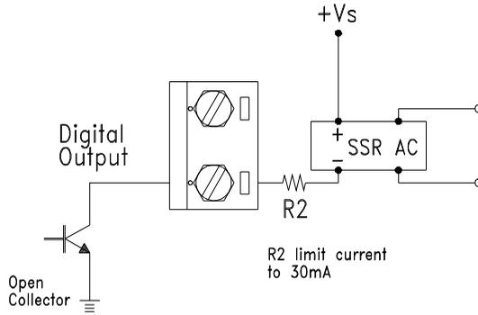
**Figure 3-6 ADAM-4011/4011D Digital Output Wiring Diagram
