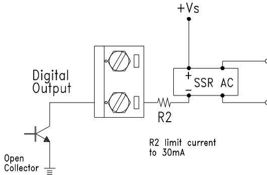
Figure 3-12 ADAM-4012 Digital Output Wiring Diagram
