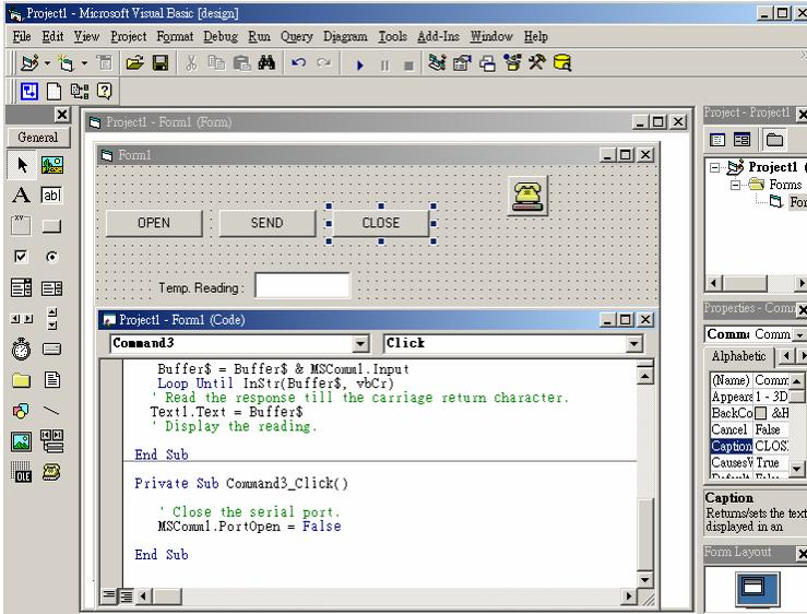
**Step 10.** Run the Project → Click OPEN to open COM1 → Click SEND to send the Get Temperature Reading Command. Now, you will find the reading the same as the displayed format shown below.
