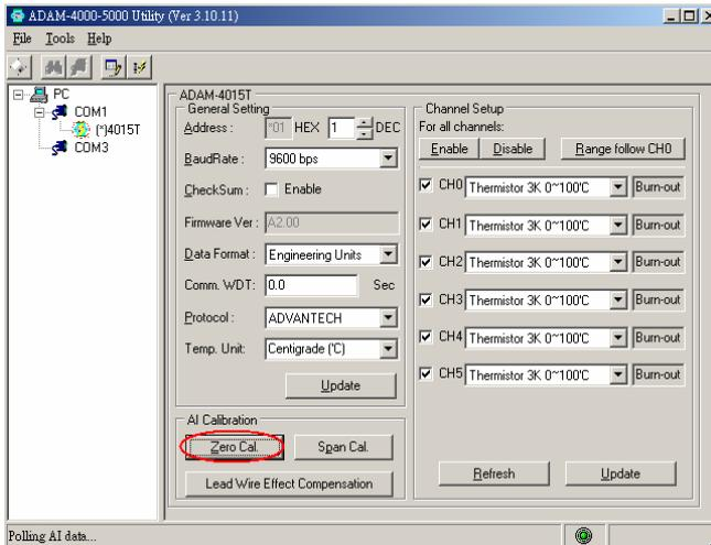
5. Apply 200.0 ohms resistor with 0.01% accuracy to CH0 and then Click on “Save”
