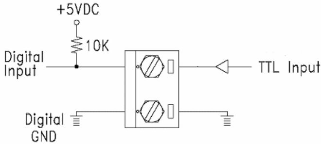
**Figure 3-7 ADAM-4011/4011D Digital Input Wiring Diagram
