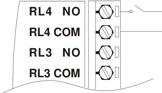
**Figure 3-66 ADAM-4068 Form A relay output Wiring Diagram**
