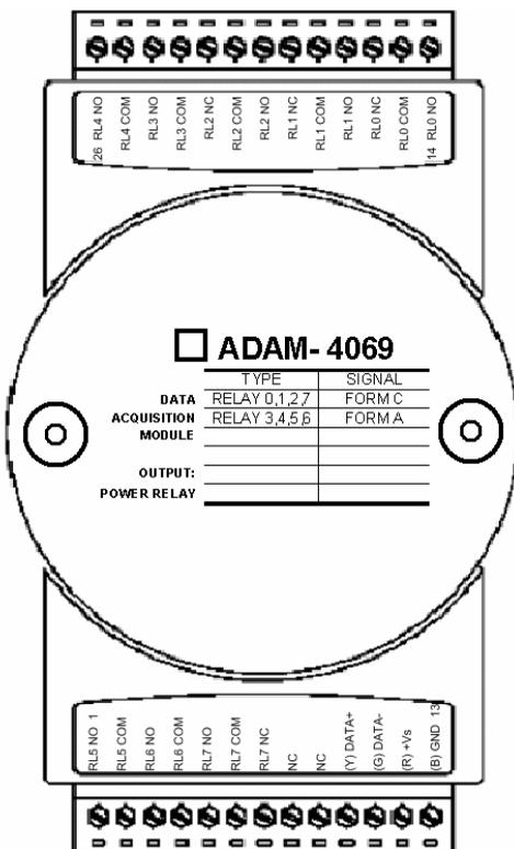
Figure 3-67 ADAM-4069 Relay Output Module
