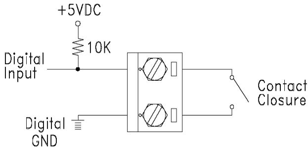
**Figure 3-8 ADAM-4011/4011D Digital Input Wiring Diagram
