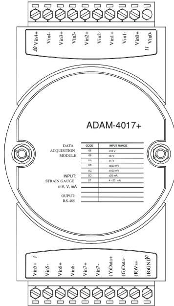
Figure 3-26 ADAM-4017+ 8-ch. differential analog input module
