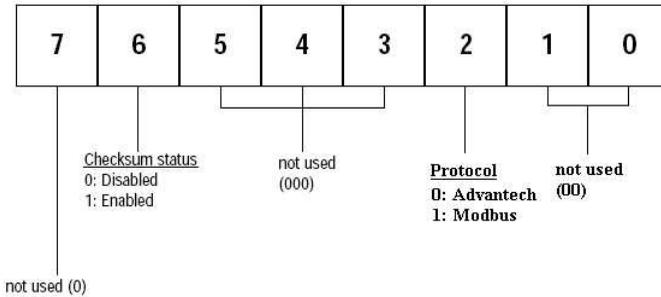
**Figure 7-2 Data format for FF (8-bit parameter)**
