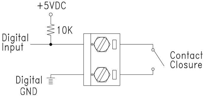
Figure 3-42 ADAM-4050 Contact Closure Input Wiring Diagram
