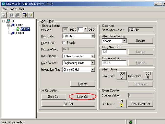
**Figure 8-3 Span Calibration**
