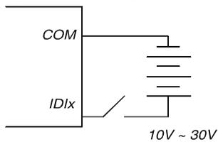
**Figure 3-39 ADAM-4024 Pin Define and Wiring Diagram**
