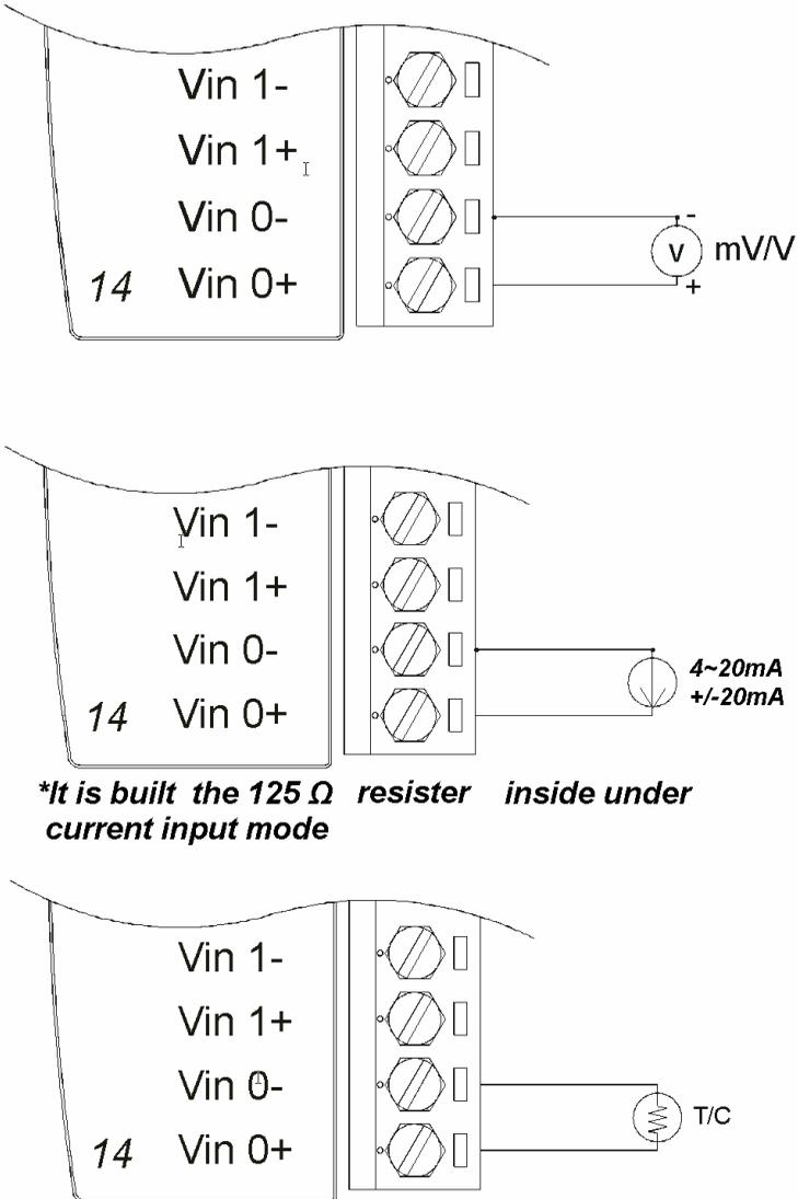
Figure 3-35 ADAM-4019+ Universal Analog Input Wiring Diagram
