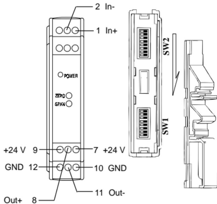
**Figure 1: Terminal Wiring Diagram**
