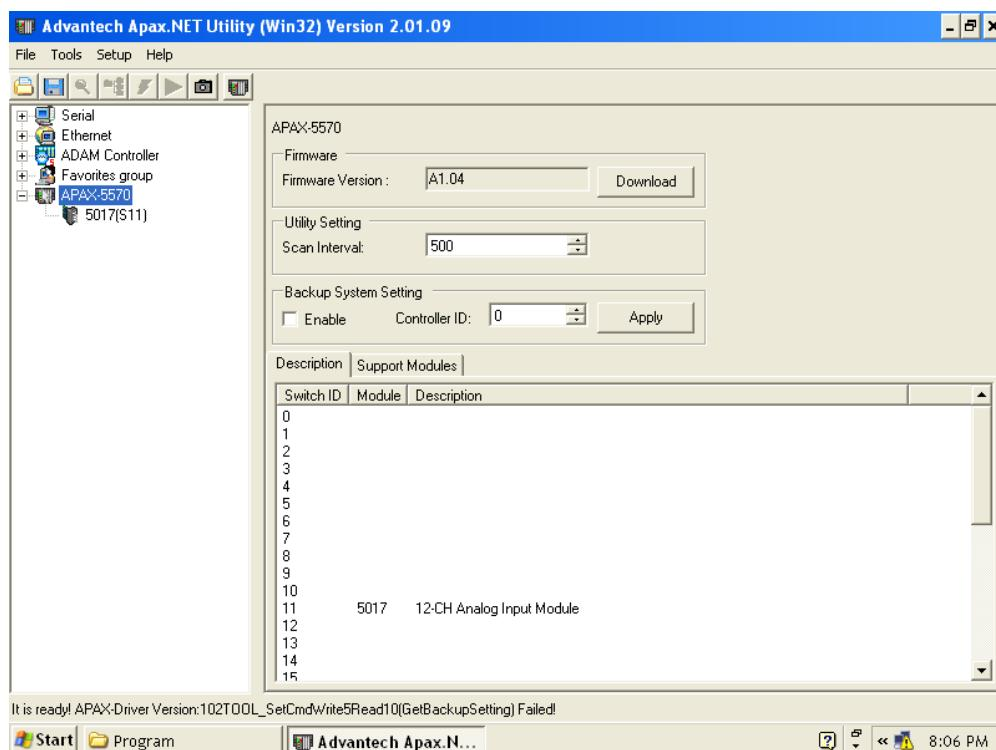
All I/O modules with its ID number are listed in the **Description** tab in the **Module Tree Display Area** (the left tab) and **Description** tab on **Status Display Area** (the right tab). You can see all I/O modules supported by APAX-557X by the **Support Modules** tab on **Status Display Area**. The **Backup Setting** check box is used to enable or disable APAX-557X backup function. Refer to Appendix C for more detail about backup functionality.
