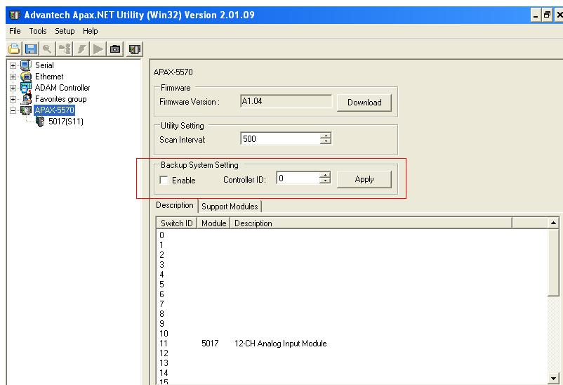
**Note!** After applying the configuration for the backup system, remember to power cycle the whole system to run the backup functionality.
