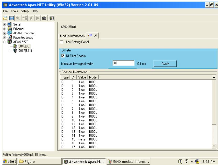
There are two parts for the **I/O Information** tab of APAX-5000 DI module. At the bottom is the **Channel Information** Area. You can see all channels' type, value, and mode. Above the **Channel Information** Area is the **Setting Panel** Area. If you don't want see the **Setting Panel** Area, you can click the **Hide Setting Panel** check box to hide the **Setting Panel** Area.
