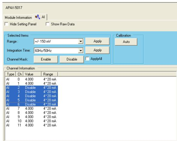
By clicking on the **Auto** button, you can perform auto calibration to the AI module. The module will automatically calibrate itself. You don't need to connect any external devices or instruments.
