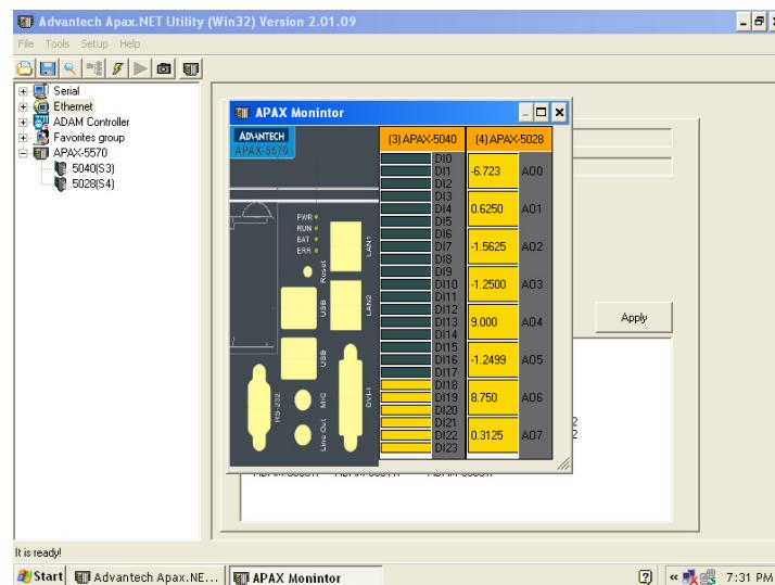
DI and AI channel values are displayed on the window. Click the DO channels to change its value. Clicking the AO channels, another pop-up window will let you configure the output value. (Refer to figure below)
