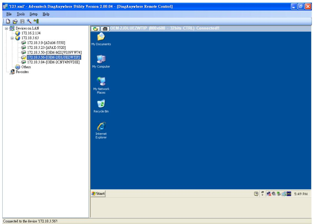
DiagAnywhere server can only run on Advantech's TPC, UNO, AMAX, APAX and ADAM Windows based devices. The supported platforms include Windows XP and Windows XPe.
