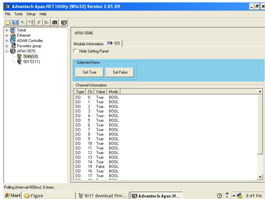
There are two parts for the **I/O Information** tab of APAX-5000 DO module. At the bottom is the **Channel Information** Area. You can see all channels' type, value, and mode. Above the **Channel Information** Area is the **Setting Panel** Area. If you don't want see the **Setting Panel** Area, you can click the **Hide Setting Panel** check box to hide the **Setting Panel** Area.
