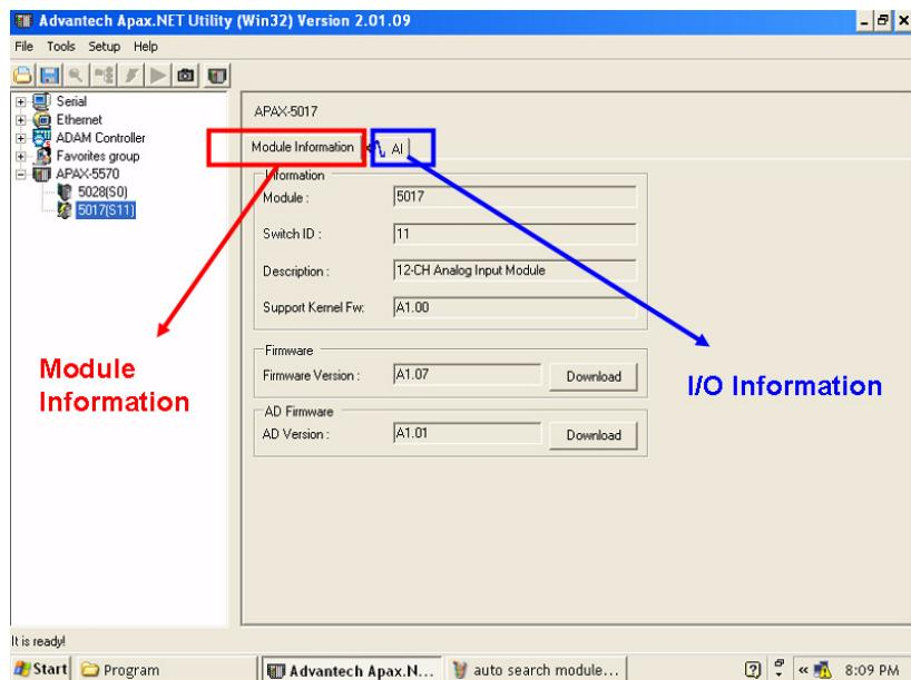
On the **Module Information** tab, module information (such as module name, switch ID, module description, and firmware version) is displayed. You also can update related firmware to the specific module by the **Download** button.
