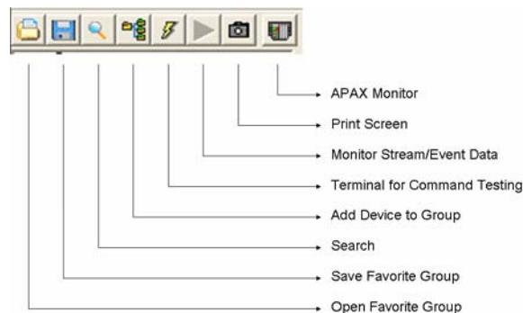
Click the **Print Screen** button, you can capture current window image of APAX.NET utility and save it to an image file. Click the **APAX Monitor** button, there will be one pop-up window showing status of all APAX-5000 I/O modules connected with APAX-557X, including ID number and channel value.
